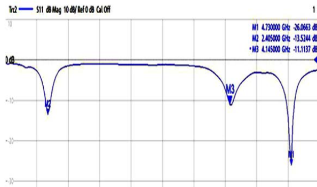
Fig. 2: Frequency vs. S11 (dB) plot of the fabricated antenna from VNA
